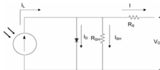
Fig. 3.2 Equivalent circuits of PY array
