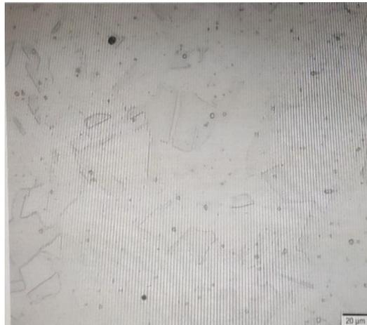
Fig.1 microstructure of 304 stainless steel
