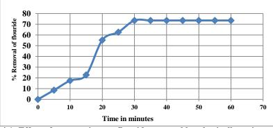
Figure 4.1: Effect of contact time on fluoride removal by physically activated carbon
