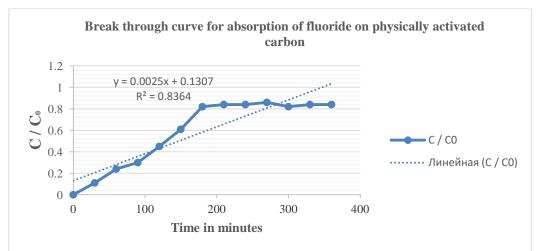
Fig. 4.26: Break Through Curve for Single Adsorption of fluoride on Physically Activated Carbon
