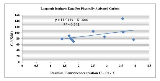
Fig.4.15: Plot of Langmuir Isotherm for physically activated carbon
