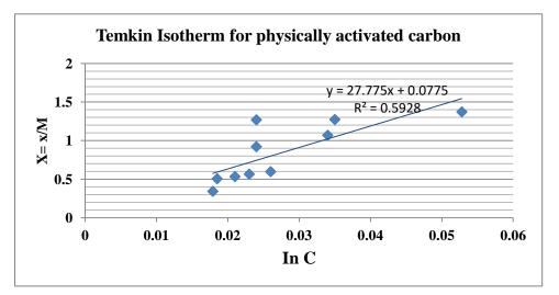
Fig.4.19 Plot of Temkin Isotherm for physically activated carbon
