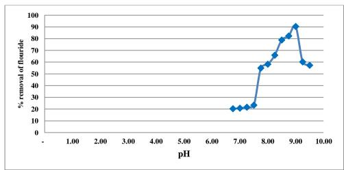
Figure 4.7: Effect of pH on fluoride removal by physically activated carbon
