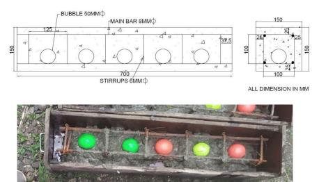
Beam Section with HDPE Ball
