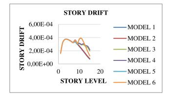
Fig 12: Drift in EQX direction
