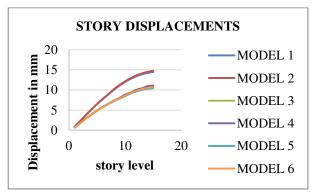
Fig 11: Displacement in WINDY direction
