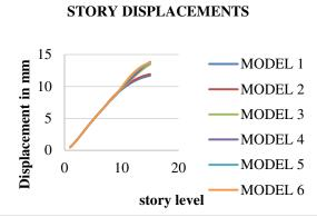
Fig 10: Displacement in WIND X direction
