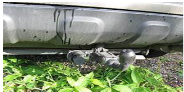
Fig(b) A trailer coupled onto a ball-type tow hitch Fig (c) A tow hook mounted on the rear of a vehicle
