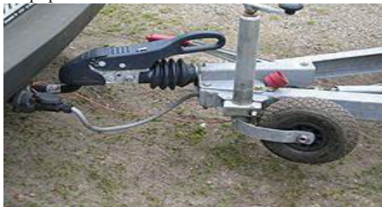
Fig(b) A trailer coupled onto a ball-type tow hitch Fig (c) A tow hook mounted on the rear of a vehicle
