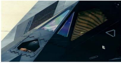
Fig.16 Reflection of F-117's Cockpit Coating (From [4])
