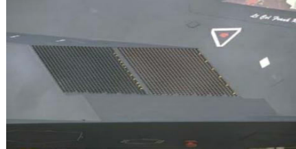
Fig.17 Thin Mesh Grid, at the Engine Intake of F-117 (From [4])
