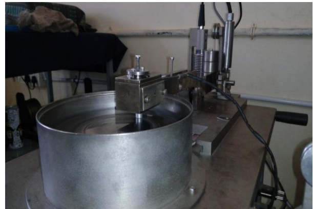
Figure 2: Wear test by pin-on-disc machine
