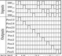
FIGURE 7. All possible combinations of a single wheel position. The positions Pos12, Pos14, Pos23, and Pos34 are sensed directly on the input of the micro-controller, while the positions Pos1 to Pos5 are determined depending on the combination of the switches Sxy activated simultaneously.
