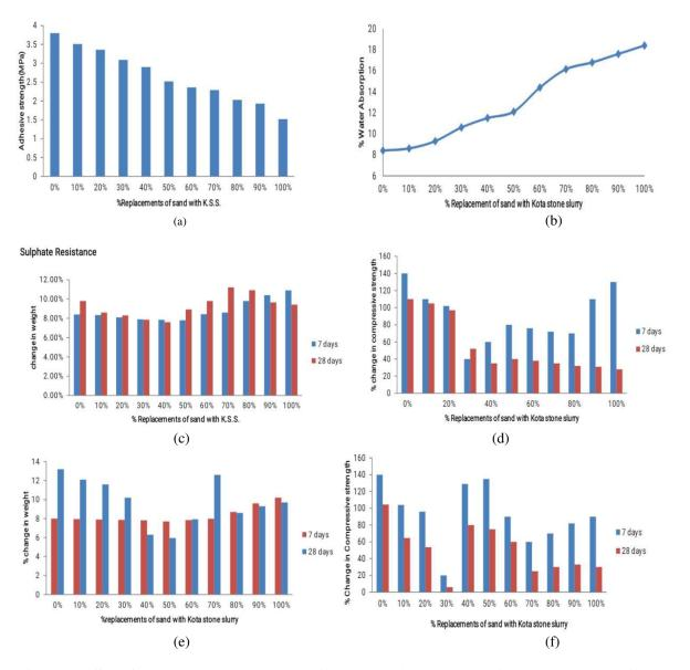
Figure 3.4 Effect of Kota stone slurry on (a) Adhesive strength, (b) water absorption, (c) Percentage weight change v/s Percentage Replacement in sulphate medium, (d) Percentage compressive strength change v/s Percentage Replacements in sulphate medium, (e) Percentage weight change v/s Percentage Replacement in Acidic medium, (f) Percentage compressive strength change v/s Percentage Replacements in Acidic medium.
