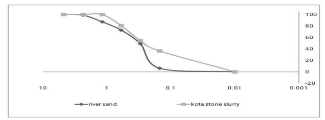
Figure 3.1 Gradation of river sand, kota stone slurry, and kota stone crushed sand
