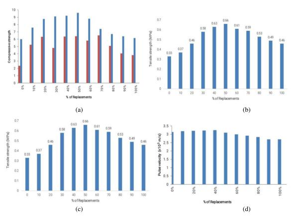
Figure 3.3 Effect of Kota stone slurry on (a) compressive strength, (b) Flexural strength, (c) Tensile strength, (d) Pulse Velocity
