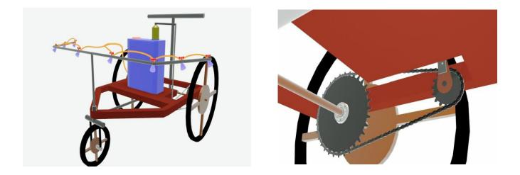
Figure (d): Assembled view of the Sprayer and power transmission
