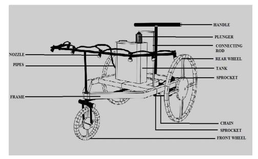
Fig (b): Parts View of the model
