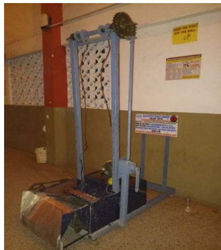
Fig.1 Semiautomatic Wall Plastering Machine
