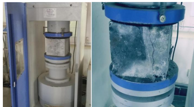
Fig: Mixing of concrete mix, Casting moulds and curing the specimens, Compressive strength of cubes
