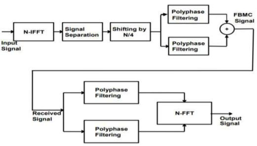
Figure 3: Simplified FBMC transceiver
