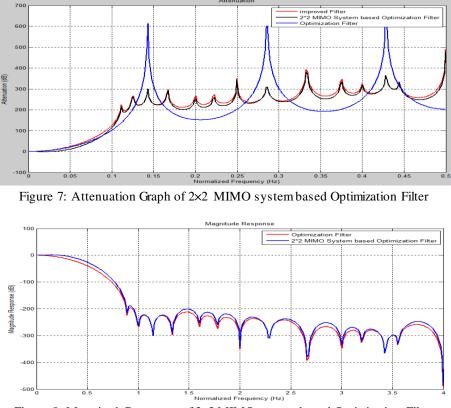
Figure 8: MagnitudeResponse of 2×2 MIMO system based Optimization Filter
