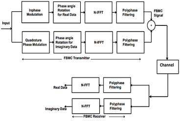
Figure 2: Block diagram of FBMC transceiver
