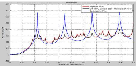
Figure 4: Attenuation Graph of 2×1 MIMO system based Optimization Filter
