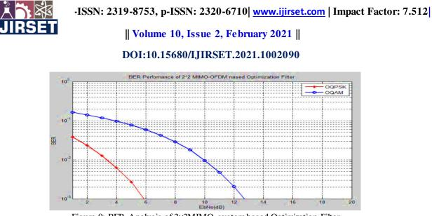
Figure 9: BER Analysis of 2×2MIMO system based Optimization Filter
