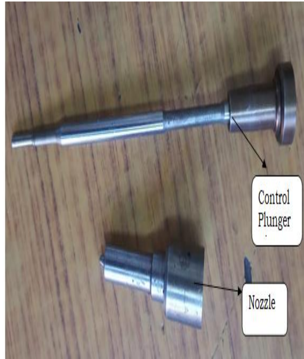
Figure 5(b): Control Plunger and Nozzle of an Injector Injector[5]
