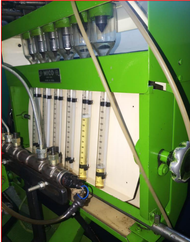
Figure 6(a): Fuel Sample collected from Main supply and Return supply of Injector
