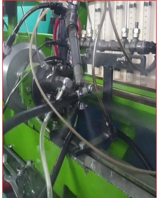
Figure 6(b): Injector with a 6 hole nozzle Spraying the Fuel
