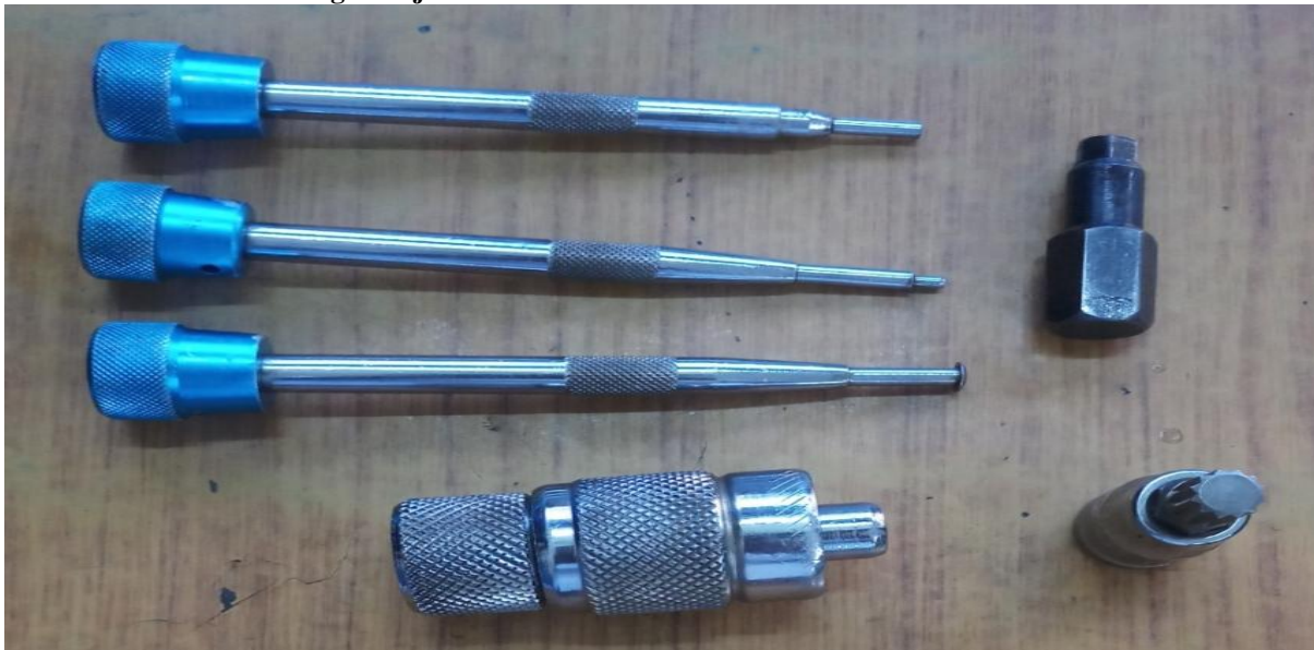
Figure 4(a): The tools used for Disassembling an Injector
