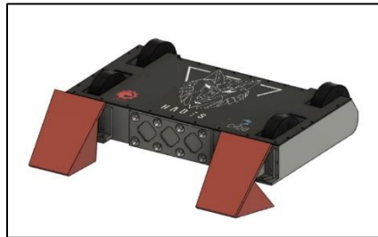
Figure 10- CAD model of 30kg defensive robot
