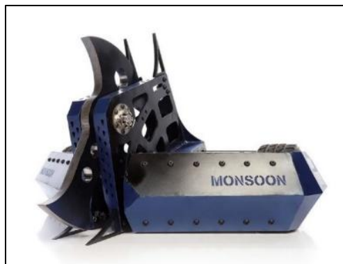
Figure 1: Monsoon, a vertical spinner with an invertible body [1]
