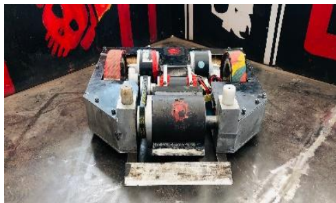
Figure 2: Centaur, a 30-kilogram drum bot
