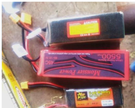
Figure 8: Different cell types of Lipo battery
