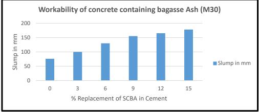
Fig. 5.2 Slumps of M-30 at different percentage SCBA
