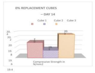
Fig. 7. Conventional cubes strength at 14 days
