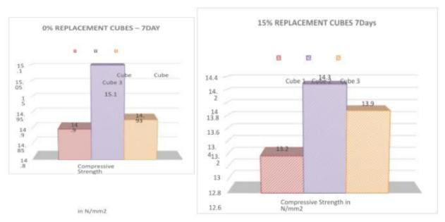
Fig.3. Conventional cubes strength at 7 days
