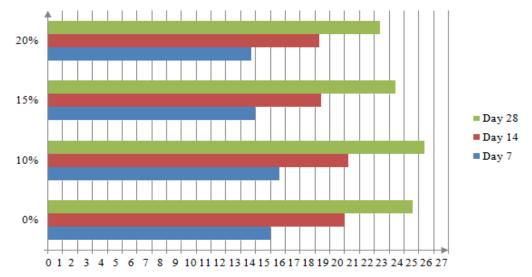
Fig.15. Combined data of all cube strength with % replacement and No of days
