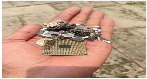
Fig.1. electronic waste as coarse aggregate
