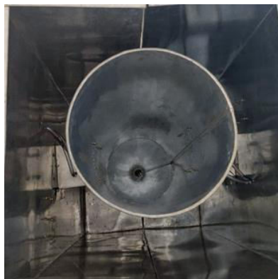
Fig.2(a) Top View of Silo Setup
