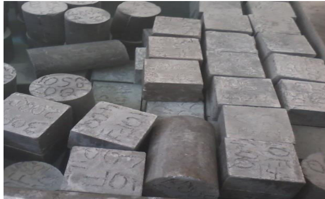
Figure 5. Specimens in Curing Tank
