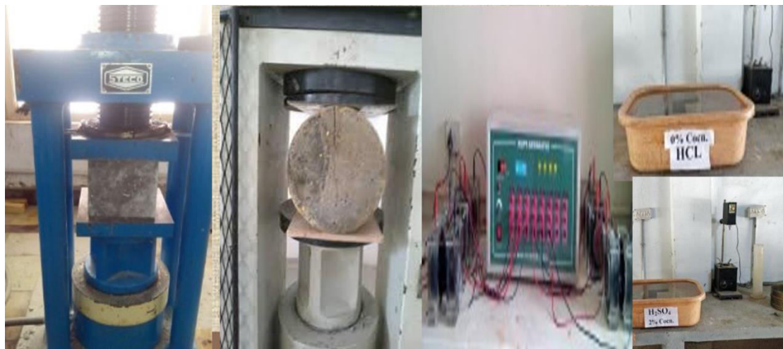
Figure 6. Tests conducted on Hardened concrete a. Compressive strength b. Split tensile strength c. RCPT Test.d. Water absorption Test.d. Acid attack test
