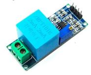
Fig.2.Voltage Sensor ZMPT101B
