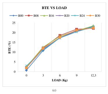
Fig. 6 Variation of BTE with load (a) CR14 (b) CR16 (c) CR18
