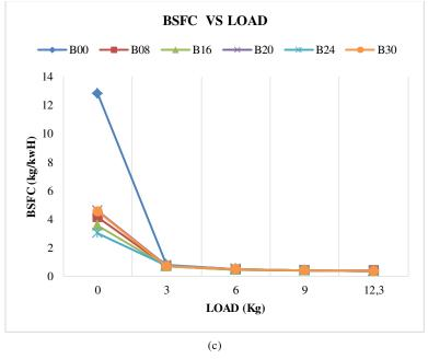
Fig. 5 Variation of specific Fuel Consumption with load (a) CR14 (b) CR16 (c) CR18
