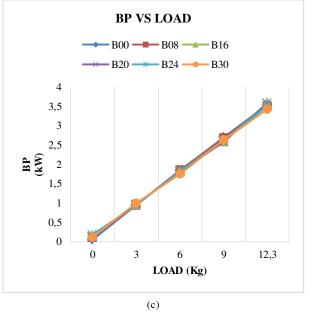
Fig. 2 Variation of BP with load (a) CR14 (b) CR16 (c) CR18
