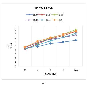
Fig. 3 Variation of IP with load (a) CR14 (b) CR16 (c) CR18
