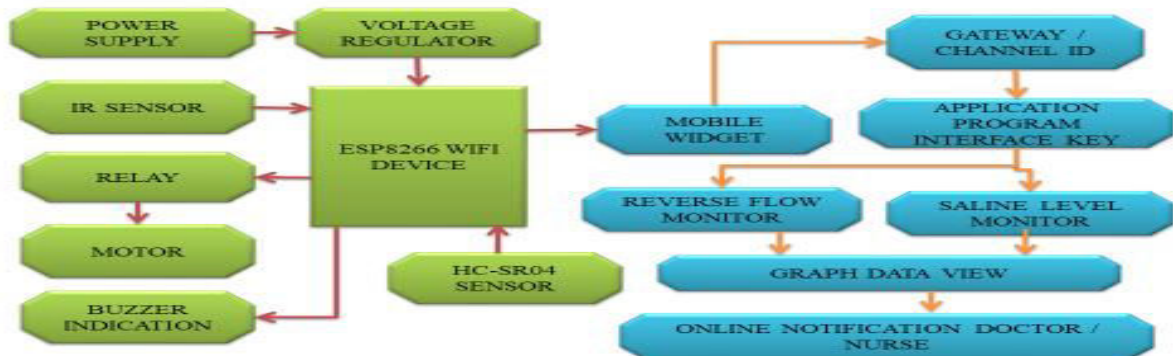
Fig. 3 Flow Diagram of the saline monitor system
