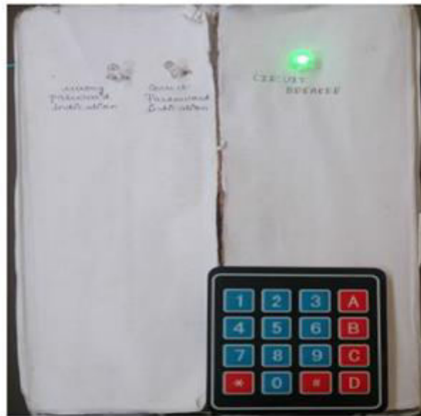
Figure 3: Front view of switchgear panel in which incomer MCCB is situated with password keypad and indication.
