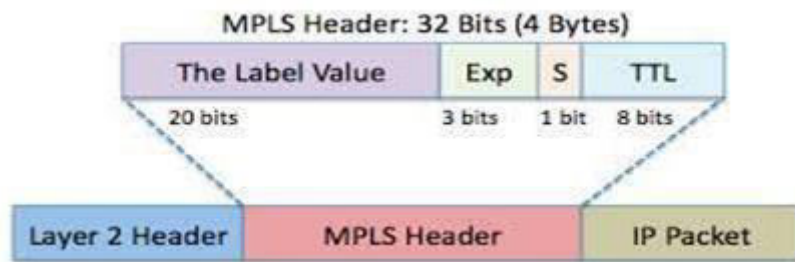
Figure 4. MPLS header
