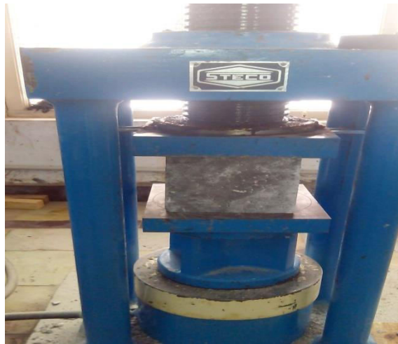
Fig5: Cube compressive strength test the above figures shows a compressive testing machine in which compressive strength of cube is being tested.
