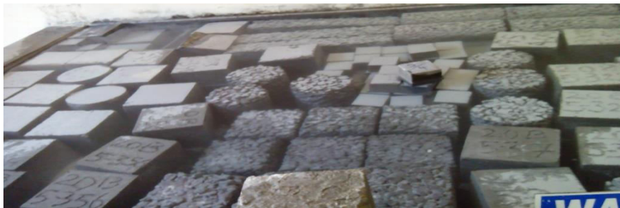
Fig4: Curing tank above figure shows a curing tank in which concrete is kept for 3, 7, 28, 56, 90 days for hydrating of concrete.
