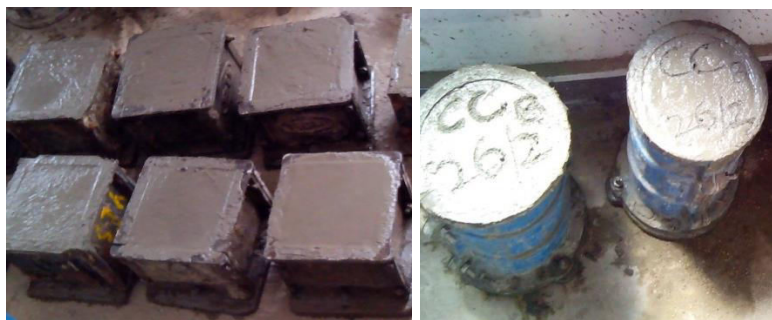
Fig 3: Sampling of concrete above figure shows casting of concrete cubes, cylinders and prisms.
