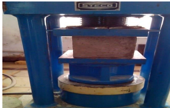
Fig5: Cube compressive strength test the above figures shows a compressive testing machine in which compressive strength of cube is being tested.
