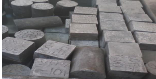
Fig4: Curing tank above figure shows a curing tank in which concrete is kept for 3, 7, 28, 56, 90 days for hydrating of concrete.
