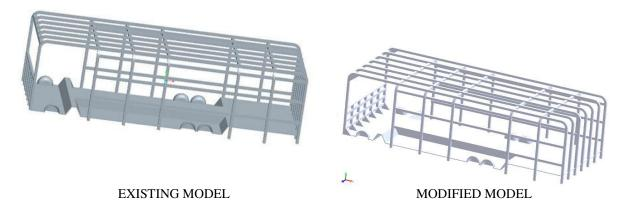
The impact analysis was carried out at 3 different speeds that is 65,140 and 200 kmph with both the models.
