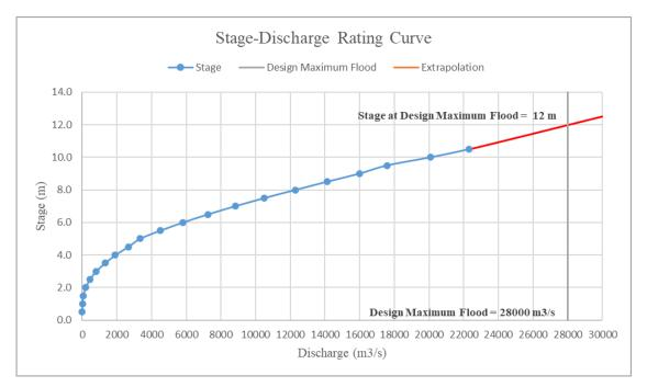
(Fig.1) Graphical illustration of Stage-Discharge Rating Curve
