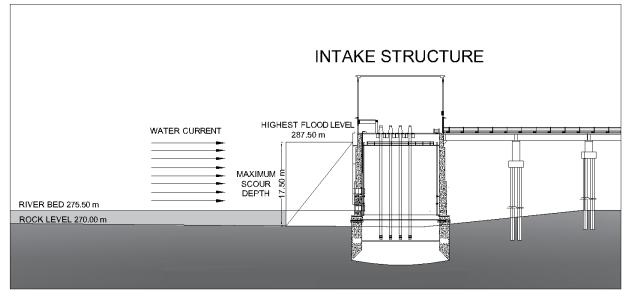
(Fig.5) River Intake Structure
