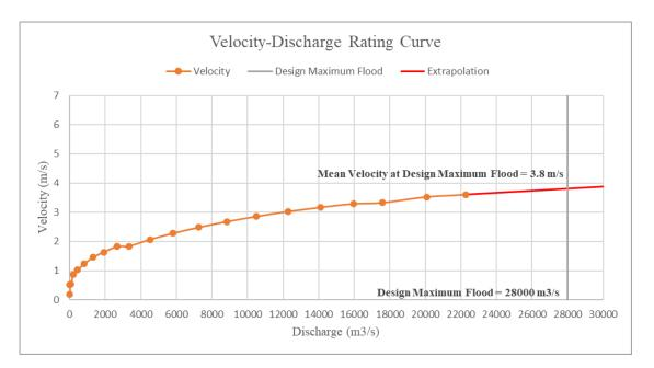
(Fig.2) Graphical illustration of Velocity-Discharge Rating Curve
