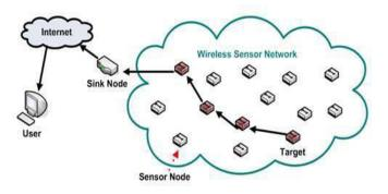
**Figure.2.Wireless Sensor Network**
