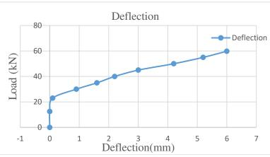
Figure 2 Load vs. Deflection Curve of CFRP Wrapped Concrete Arch
