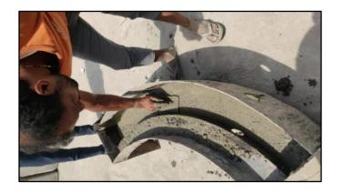
Figure 1a Casting of Specimen
