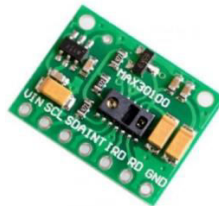
Fig. MAX30100 Pulse Oximeter Heart Rate Sensor Module
