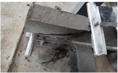
Figure 3a Failure pattern of Reinforced Concrete Beam
