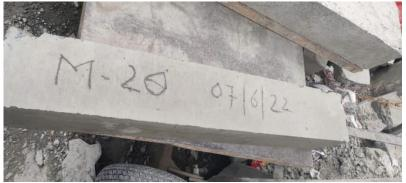
Figure 1aRCB specimen after 28 days curing period
