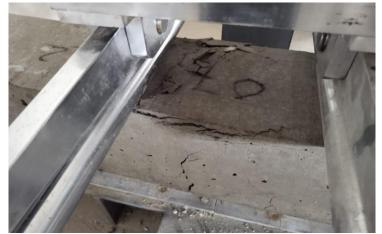
Figure 3b Failure pattern of Reinforced Concrete Composite Beam-1
