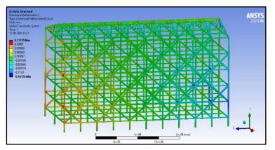
Figure 2 shows the displacement in Z direction the maximum displaced values is +0.1311mm and -0.1412mm both are similar but opposite in direction and the minimum displaced value is 0.0100mm.
