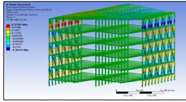
**Figure 1 Displacement in X-Directions**
