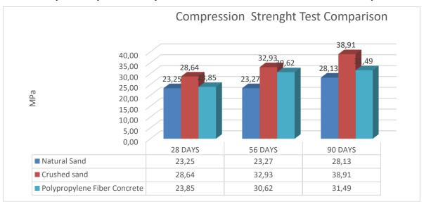
Graph 03 Comparison of Compression Test of Mix M1, M2, And M3 for 28, 56 & 90 days.
