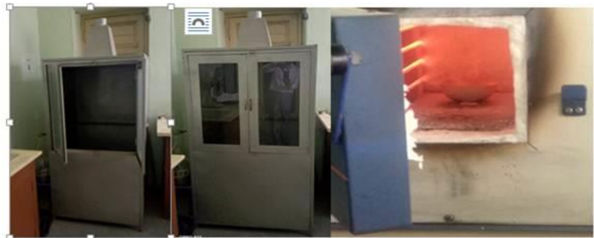
Figure 4. Fabricated chamber & furnace used for combustion synthesis.
