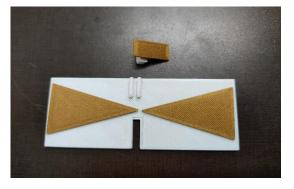
Fig 5.3.4: Printed Backscattering antenna.
