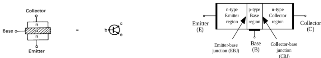
Figure 1: To the left, the three different electrodes are specified in the first two. The last figure to right is commonly used as a symbol of a NPN transistor incircuit.
