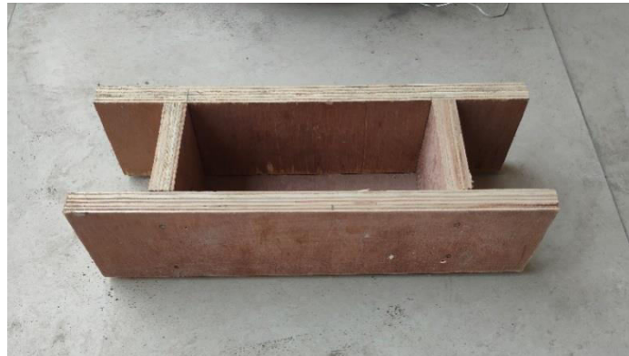
Figure 6: Mould for making brick
