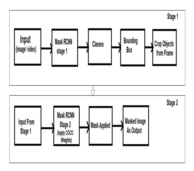
Figure.1.Block Diagram for Realtime and Video Segmentation
