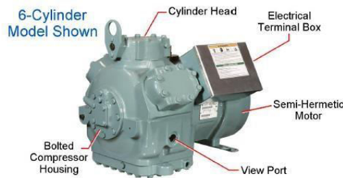
Fig.reciprocating compressor
