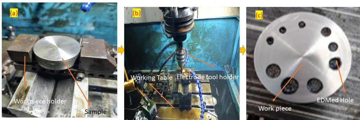
Figure 1. EDM setup with workpiece (a) Circular workpiece with workpiece holder, (b) EDM tool holder with workbench, (c) final machined workpiece.
