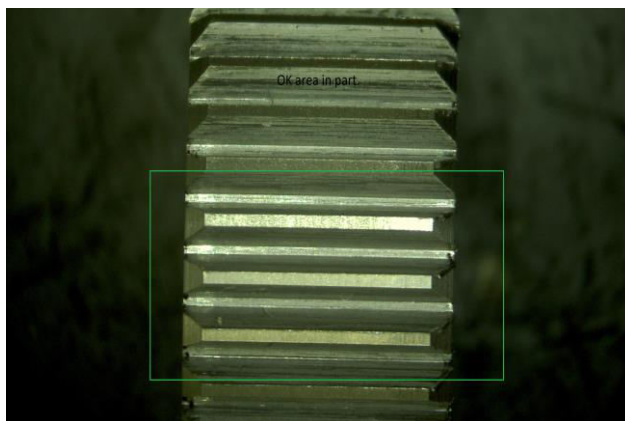
Fig. 7 Gear with burr Free (ok)
