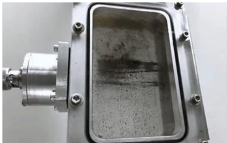
Figure (13)- Particles being suspended an account of acoustic forces.
