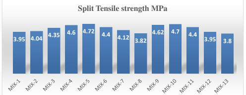
FIG 8. Graphical representation of Split Tensile strength of various mix of CC concrete and Fibrofor fiber concrete.
