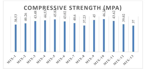
FIG 7. Graphical representation of Compressive strength of various mix of CC concrete and Fibrofor fiber concrete.
