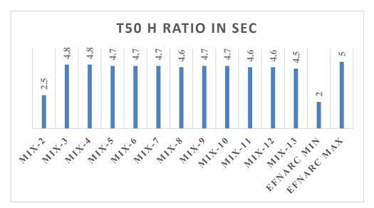
FIG 3. Graphical representation of T<sub>50</sub> H ratio in sec of various mix of CC concrete and Fibrofor concrete.
