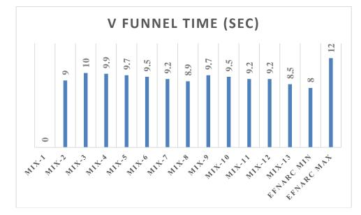
FIG 4. Graphical representation of V-Funnel time in seconds of various mix of CC concrete and Fibrofor concrete.
