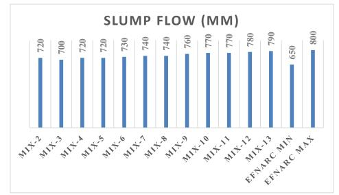
FIG 2. Graphical representation of Slump flow in mm of various mix of CC concrete and Fibrofor concrete.
