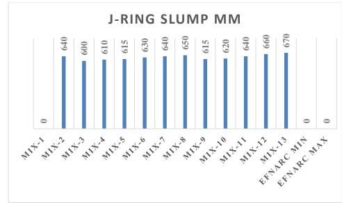
FIG 5. Graphical representation of J Ring slump in mm of various mix of CC concrete and Fibrofor concrete.
