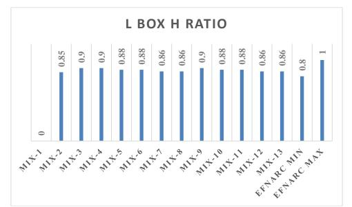
FIG 6. Graphical representation of L Box H Ratio of various mix of CC concrete and Fibrofor concrete.
