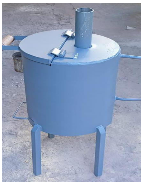
Figure4: completed model of the incinerator
