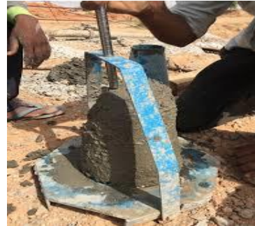
Placing a Concrete on Slump mould with adding of Fly-Ash & Coconut Fibre
