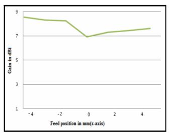
Fig. 4: Gain variations of microstrip antenna
