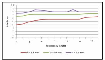
Fig. 6: Gain variations of microstrip antenna
