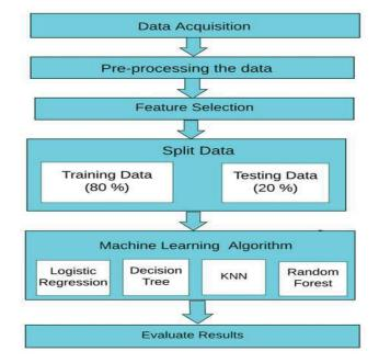
Fig. 5.1. Architecture Diagram
