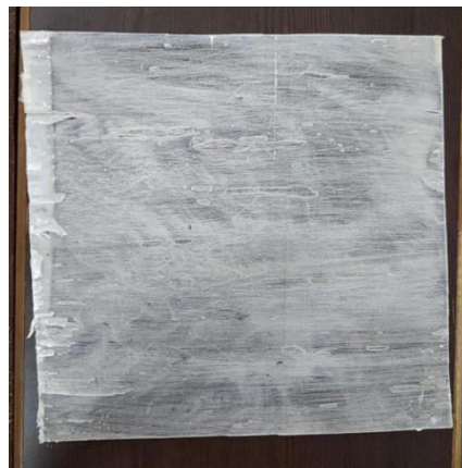
FIG BAMBO FIBER REINFORCED COMPOSITE SHEET
