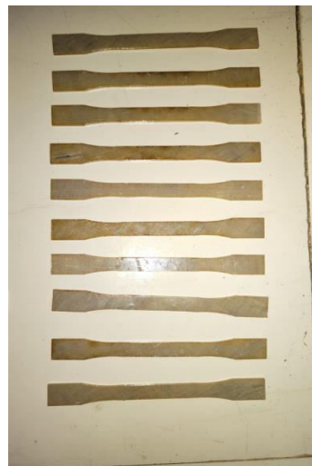
FIG ASTM D638 COTTON FIBRE SAMPLE
