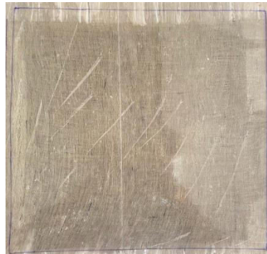
FIG COTTON FIBER REINFORCED COMPOSITE SHEET
