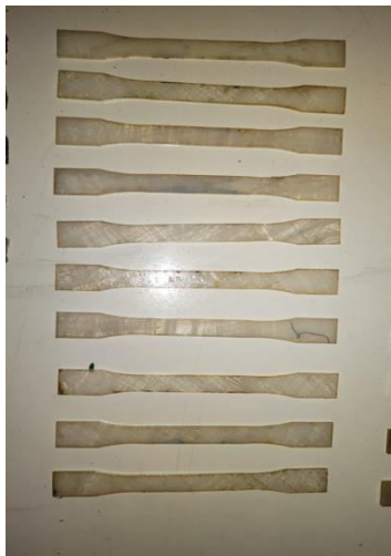
FIG ASTM D638 BAMBOO FIBRE SAMPLE
